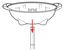
Place grease tray securely into position inside grill base. When properly placed, it is held firmly with pointed end in centre of grill base.
